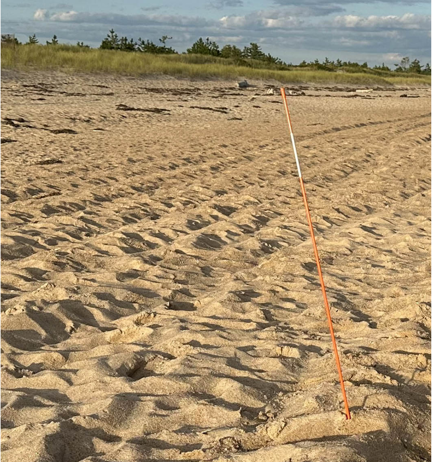
A stake placed by coastal geologist Janet Freedman marks the line between wet and dry sand. This boundary is used to measure 10 feet from the seaweed line if that is not visible, or in this case, unusually high because of storm surge. (Cynthia Drummond/Rhode Island Current)
